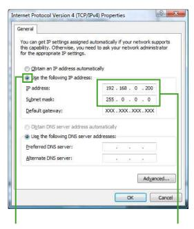
Click the [Use the following IP address] radio button and type the IP address and Subnet mask.
